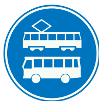
F17 Carriageway or lane exclusively for the use of line buses and trams
