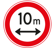
C17 Closed to vehicles Vehicles and combinations of vehicles that, including cargo, are longer than indicated on the sign
