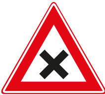
J8 Dangerous intersection
