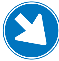
D2 Mandatory for all drivers to pass the sign on the side indicated by the arrow
