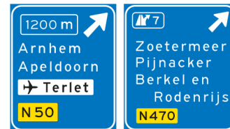
K2 Advance sign along the motorway for the exit direction, with distance indication, exit number, interlocal destinations, reference to airport/airfield, and non-motorway route number
