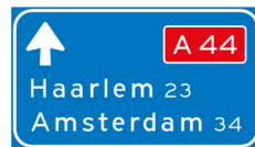
K1 Low decision directional sign along motorway for through direction, with interlocal destinations and route number motorway
